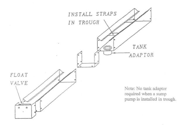
Place the mastic strips inside of the u connector and bolt together with the trough.
